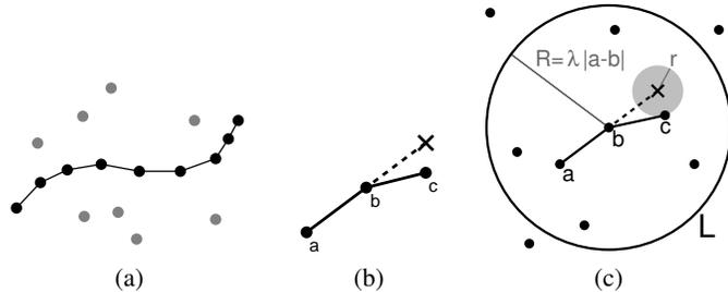
Figure 1: Definition of the *good continuation* event. (a) A candidate *chain* is defined by an ordered sequence of points. (b) Three consecutive points in a chain define a *triplet*. The ideal symmetric point is represented by X. (c) The symmetry precision of a triplet is measured by the distance  $r$  from the third point  $c$  to the ideal point  $X$ , relative to the area of the local observation window  $R$ .
