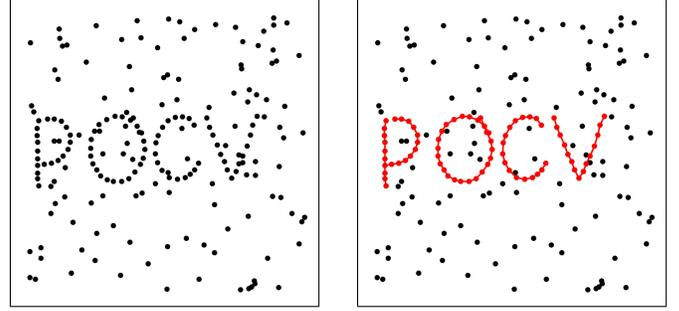
Figure 2: Result of our unsupervised perceptual grouping algorithm. **Left:** 80 points forming the word “POCV” plus 100 random points. **Right:** Detected sets of points in “good continuation”. The method automatically discovers the number of salient structures, and is able to distinguish structure from noise.
